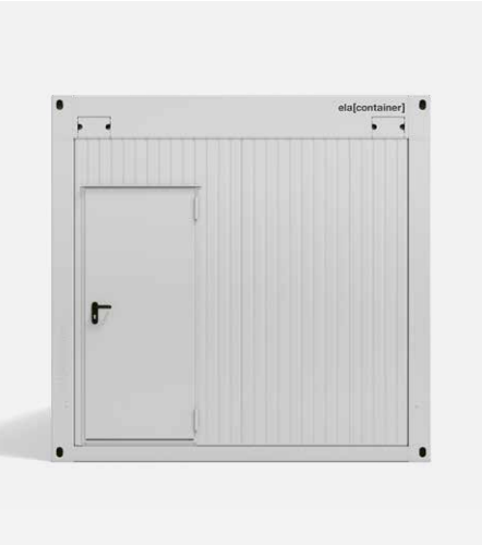
Multipurpose exterior door, 875×2,000 mm Stable, galvanised double-walled doors with lock and handle set, heavy construction hinges that comply with DIN 18272 and aluminium run channel.
